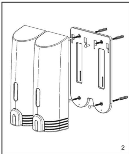
Put the rear cover on the wall, mark the location of the install hole. Drill the 4- $\varnothing$ 6mm hole according to the mark., use the screw with this product to fix the rear cover on the wall.
