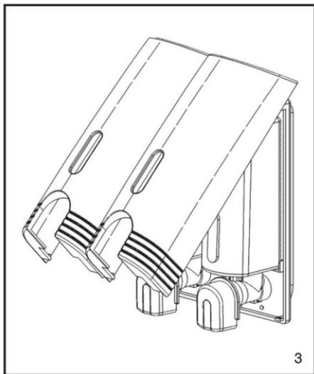
Hold the base clawing back on rear cover, open the front cover, take out the soap dispenser bottle, close the bottle cap after injection the liquid soap, fix the soap dispenser body on the rear cover.
