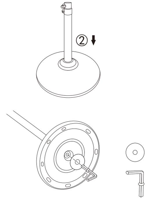
Put the lower tube into the counterweight base ,
